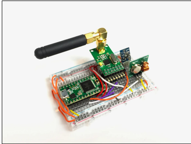
Figure 8: Device used for RollJam attack
