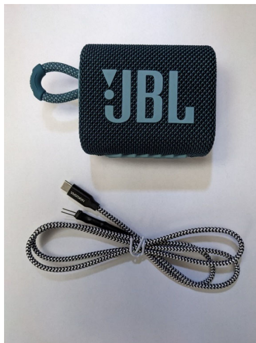
Figure 13: A CAN Injection device masked as a JBL Speaker
